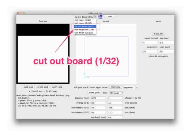
Change parameters. Set "bottom Z (mm)" and "cut depth (mm)" to -5.0 and 1.2 respectively.
